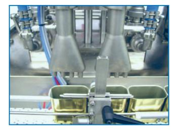
The 620 Series also includes filling machines equipped with slat conveyors for container supply and collection. One example of this setup includes units with scrolls for transportation of glass jars. Depending on the production size these filling systems are designed with between one and eight filling heads, while the glass jars are moved in either one or two lane batches.
